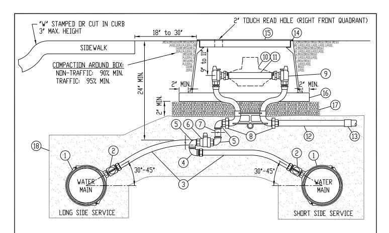
CARSON 1220-4B "T" TYPE LID: SHALL INCLUDE STRAIGHT TYPE HEXAGON LOCK-DOWN BOLT (1) AND TOUCH READ HOLE. SHALL BE MARKED "WATER"
