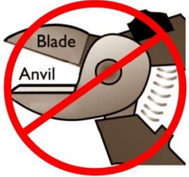
ANVIL PRUNER A single blade slices onto a flat "anvil"
