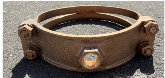
Cast iron saddle removed from service
