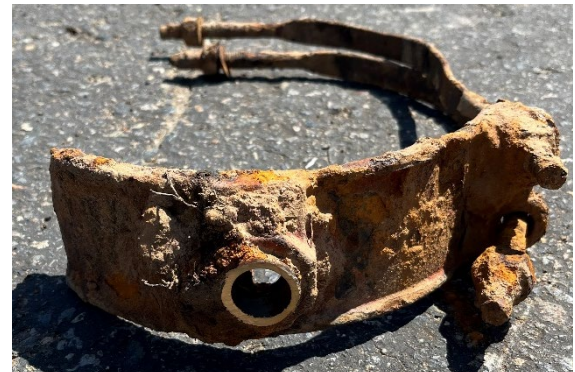
Cast iron saddle removed from service
