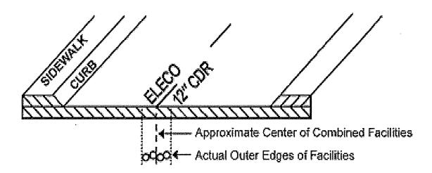
3. Changes in direction and lateral connections are clearly indicated at the point where the change in direction or connection occurs, with an arrow indicating the path of the facility. A radius is indicated with marks describing the arc. When providing offset markings (paint or stakes), show the direction of the facility and distance to the facility from the markings.
