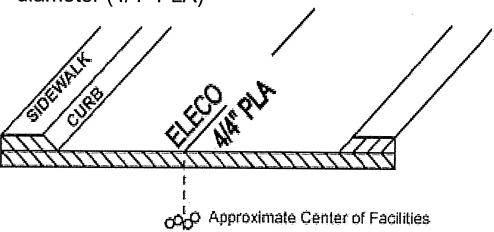
c. **Conduit Marking:** Used for any locatable facility being carried inside conduits or ducts. The marks indicating the outer extremities denote the actual located edges of the facilities being represented.
