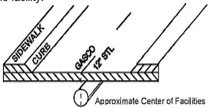
or 2) placing the marks over the approximate outside edges of the facility with a line connecting the two horizontal lines (in the form of an H) to indicate there is only one facility:
