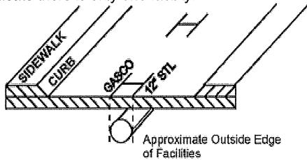
These examples indicate an operator's 12 in. facility. When a facility can be located or toned separately from other facilities of the same type, it is marked as a single facility. 2/2
