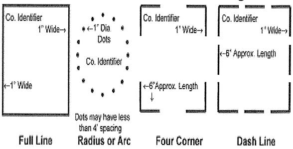
Delineate in white paint the proposed area of excavation using a continuous line, dots marking the radius or arcs, dashes marking the four corners of the project, or dashes outlining the excavation project. Limit the size of each dash to approximately 6 in. to 12 in. long and 1 in. wide with interval spacing approximately 4 ft to 50 ft apart. Reduce the separation of excavation marks
