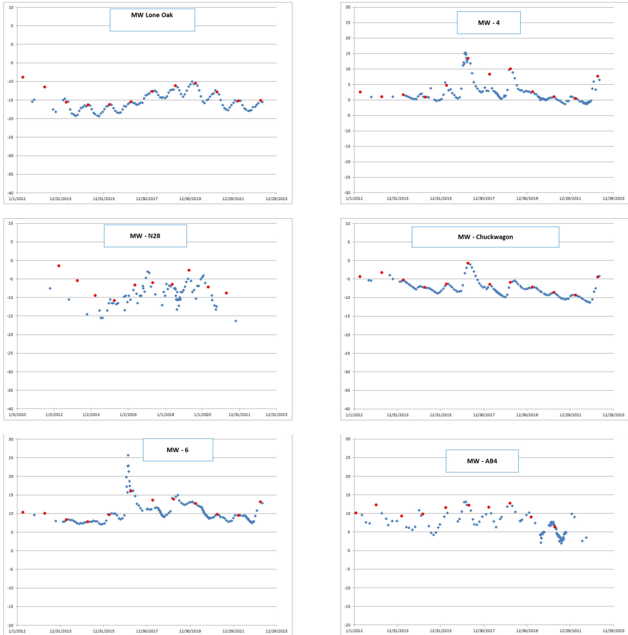
FIGURE 3-1. HYDROGRAPHS FOR BASIN MONITORING
